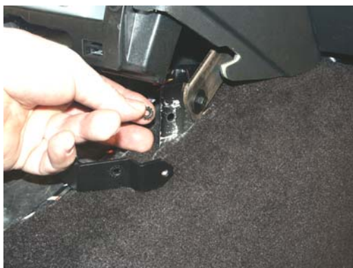
Attach passenger side, and tighten hardware on both sides (Item 2, 7, 8, 9)
